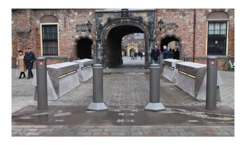
Image above illustrates possible surface finish – bollards above are weathering steel which is designed to rust. Below are stainless steel bollards with steel plate surface.
